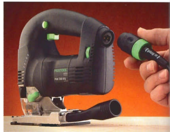
Festool's "Plug It" detachable cord is just one of many features included standard with the saw. This is a tool with no weaknesses.
