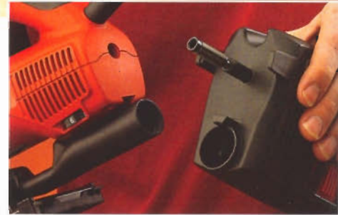
The Hilti has a cool dust collector unit. It's powered by an armature that connects to the motor via an entry hole at the back of the saw.
